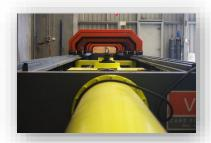
The Test Bench capabilities include proof load testing, break load testing, and low cyclic testing of steel wire ropes, chains, spreader beams, webbing slings, shackles, etc. The machine uses a hydraulic cylinder to load, a load cell to measure the testing force, and an encoder to measure the piston displacement.
