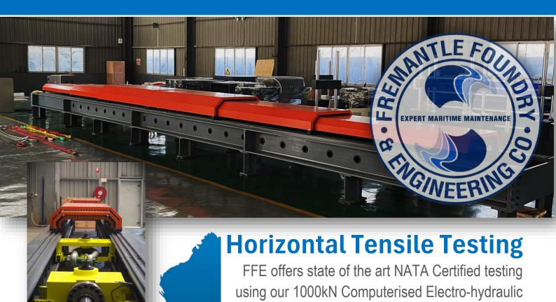
Load testing is fast and control-accuracy is high through a digitally controlled, closed-loop electro-hydraulic system and valve. Using the latest Windows technology the computer system collects and processes data to display real-time results for testing force and testing curve.
