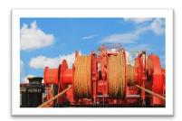
Mooring winch brake rendering tests are mandatory in the Port of Fremantle, at intervals not exceeding 24 months, and tests must be carried out in accordance with ISO Standard 3730:2012 and the latest edition of the OCIMF - Mooring Equipment Guidelines. FFE tests to these standards and issues NATA endorsed certificates with detailed reports for all mooring winch brake rendering tests.
